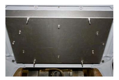
5. Place the #2 shield on the four threaded studs, paying attention to it's orientation (UP and arrow). Turn a ½-20 nut on to each stud leaving approximately ½" of stud (5-6 threads) exposed below the nut.
