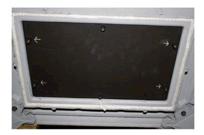
3. Insert the 4  $\frac{1}{4}$ -20 x 1 3/4" long threaded studs into the front and rear holes on the bottom of the stove's base. Snug them up with a 1/8" allen wrench.
